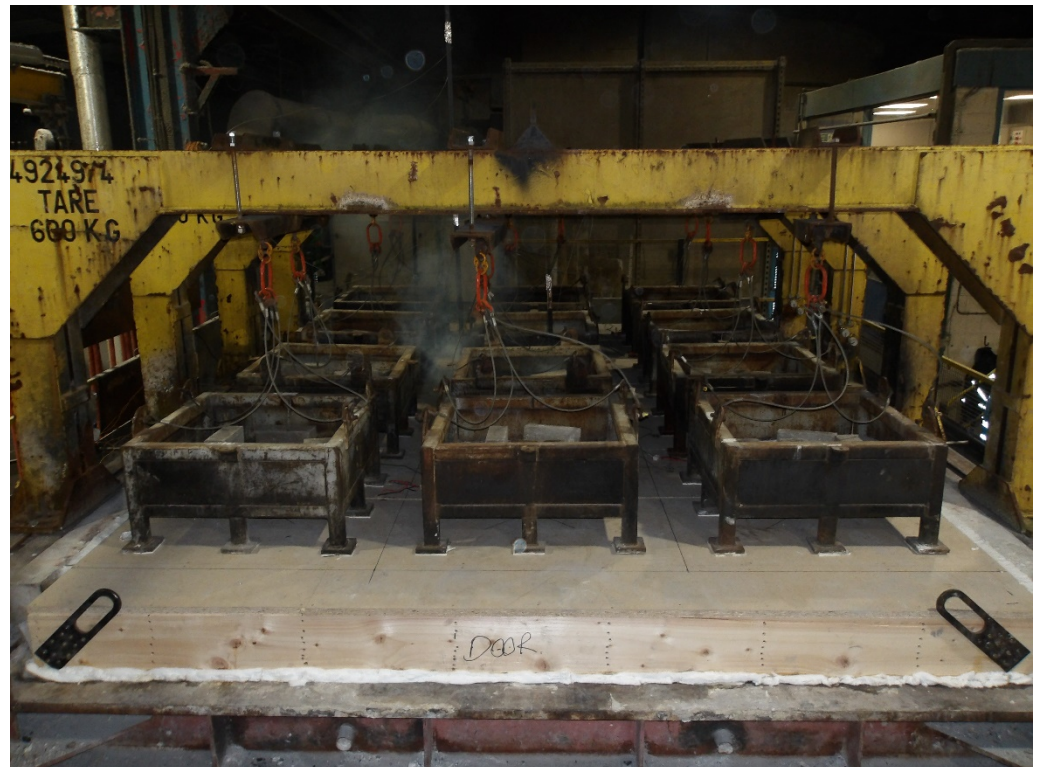
The unexposed face of the floor assembly after 90 minutes of testing
