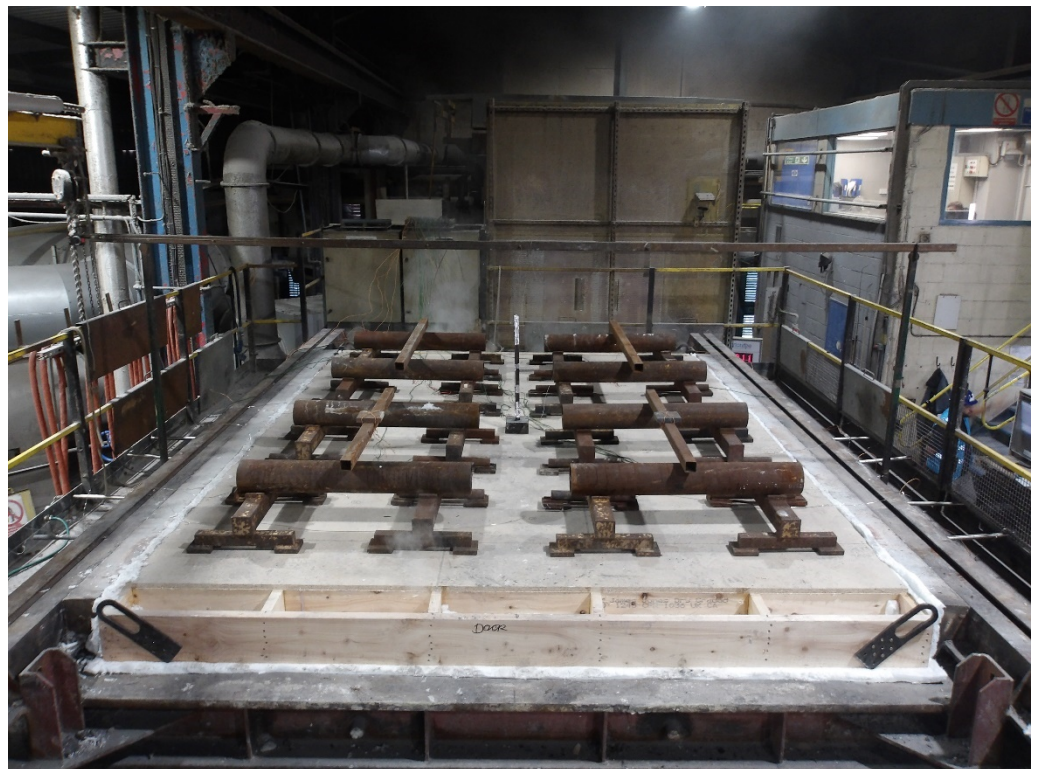
The unexposed face of the floor assembly after 40 minutes of testing
