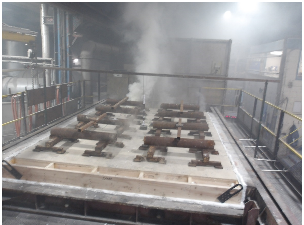
The unexposed face of the floor assembly after 70 minutes of testing
