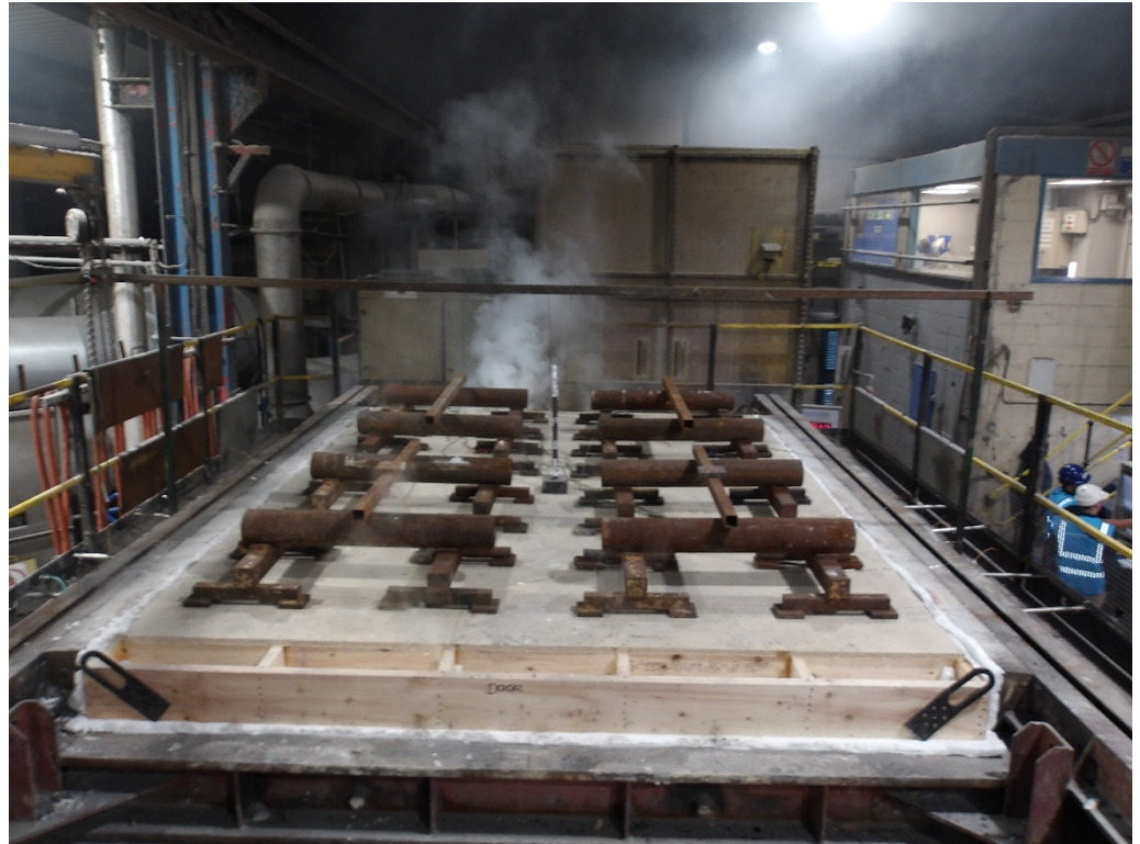
The unexposed face of the floor assembly after 60 minutes of testing
