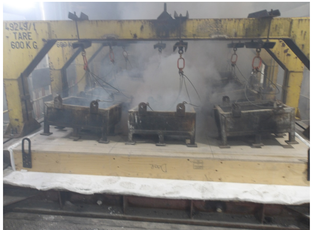
The unexposed face of the floor assembly after 35 minutes of testing
