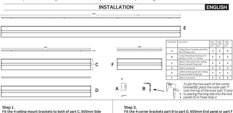
Fit the 4 ceiling mount brackets to both of part C, 600mm Side panel or 8 brackets to part E 1200mm Side panel with Ceiling Mount bracket fixing hole.
