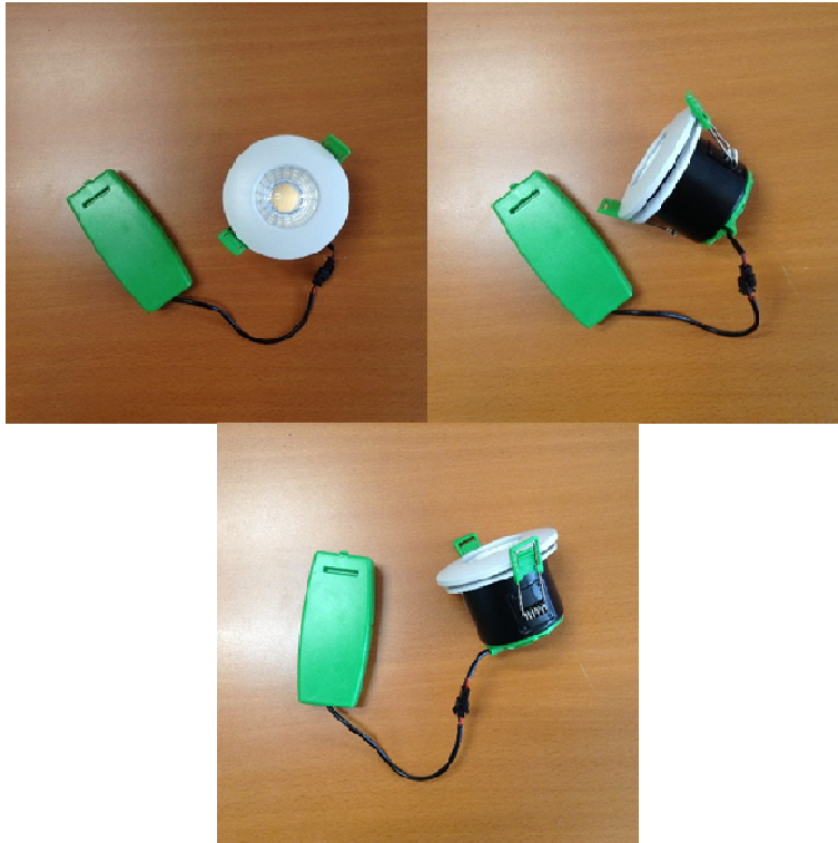
Figure 3: Photographs of the test sample: JCC Lighting Products Ltd downlight (JC1001).
