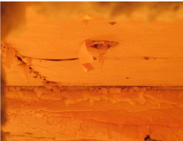
Photo 19: The exposed surface of the specimen after test duration of 45 minutes, showing the first layer plasterboard ceiling started to sag slightly and joints began to open
