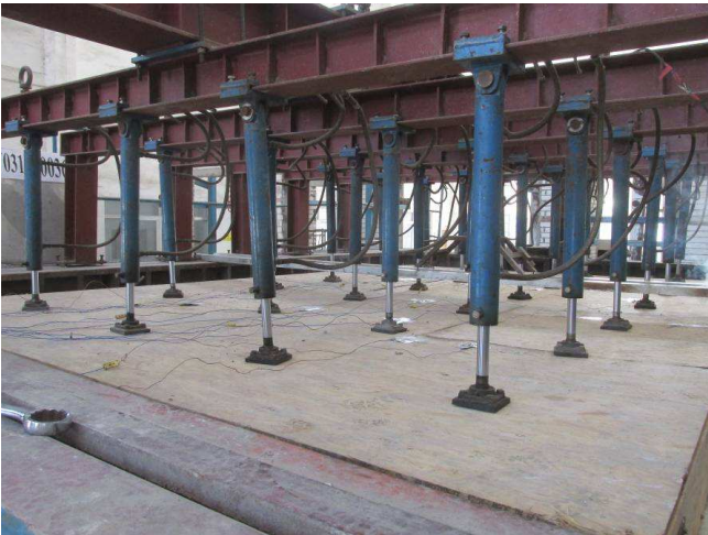
Photo 17: The unexposed surface of the specimen after test duration of 30 minutes
