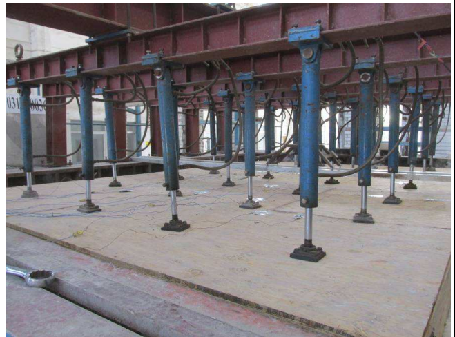
Photo 20: The unexposed surface of the specimen after test duration of 60 minutes
