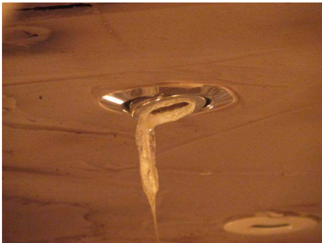
Photo 13: The exposed surface of the specimen after test duration of 2 minutes, showing the lens of specimen was fusing
