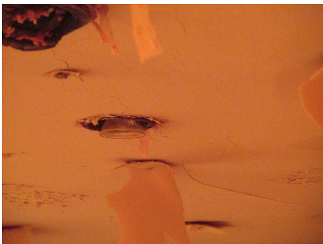
Photo 15: The exposed surface of the specimen after test duration of 22 minutes, showing the lamp cup of specimen fell out from the light can
