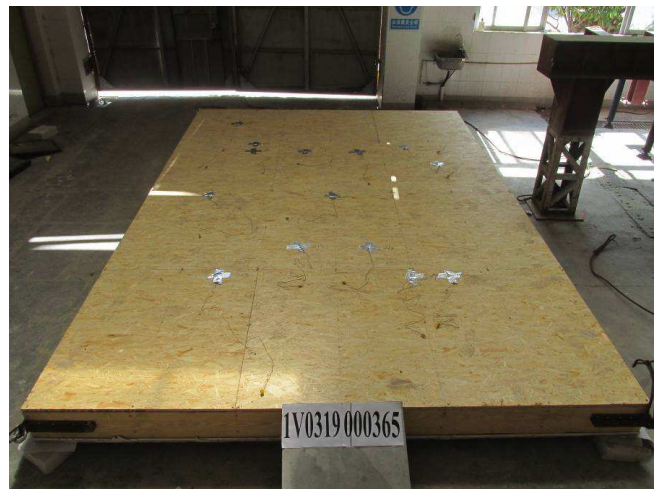
Photo 12: The unexposed surface of the specimen before the test
