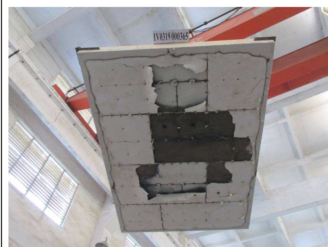
Photo 21: The exposed surface of the specimen after the test
