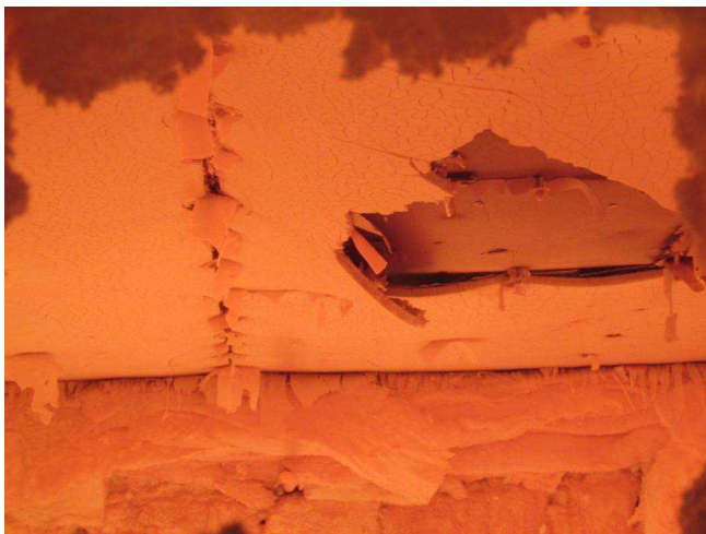
Photo 19: The exposed surface of the specimen after test duration of 57 minutes, showing part of first layer plasterboard ceiling was falling into the furnace.
