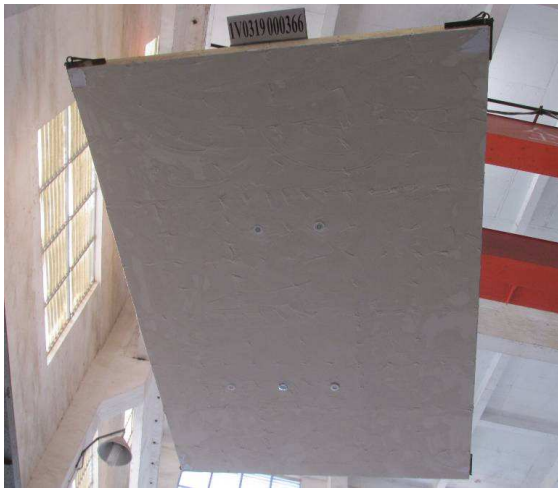
Photo 11: The exposed surface of the specimen before the test
