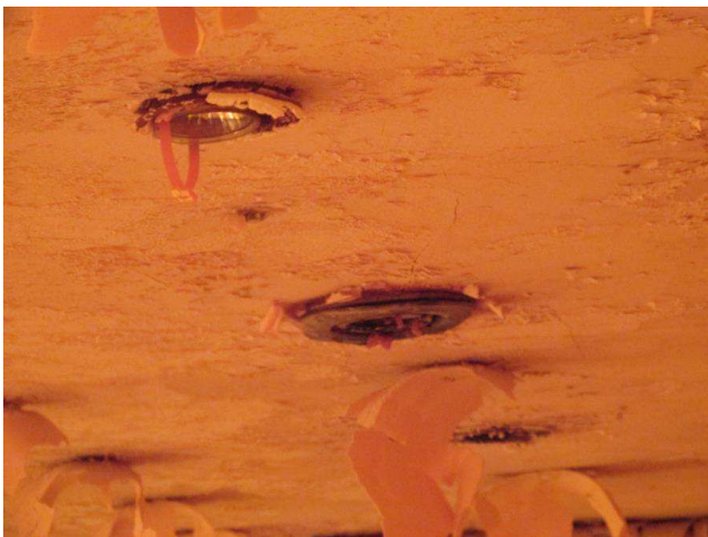
Photo 15: The exposed surface of the specimen after test duration of 16 minutes, showing the bezel of specimen fused
