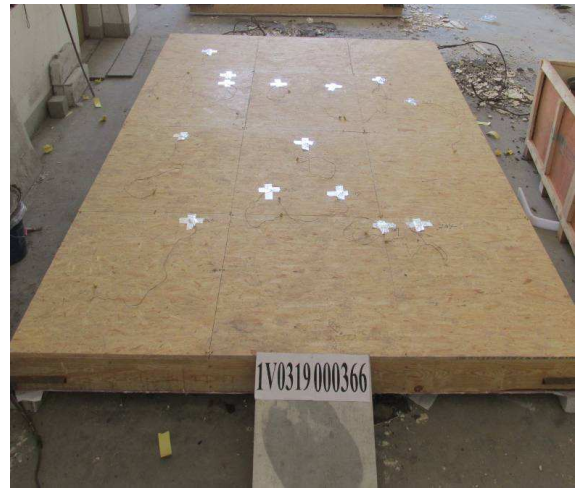
Photo 12: The unexposed surface of the specimen before the test.
