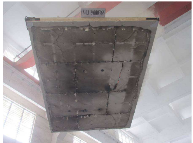
Photo 18: The exposed surface of the specimen after the test.
