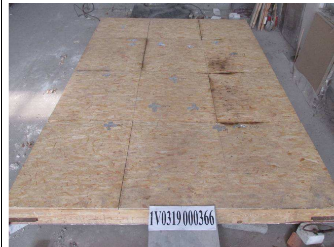
Photo 19: The unexposed surface of the specimen after the test
