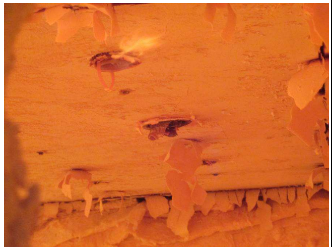
Photo 16: The exposed surface of the specimen after test duration of 22 minutes, showing the lamp cup of specimen fell out from the light can
