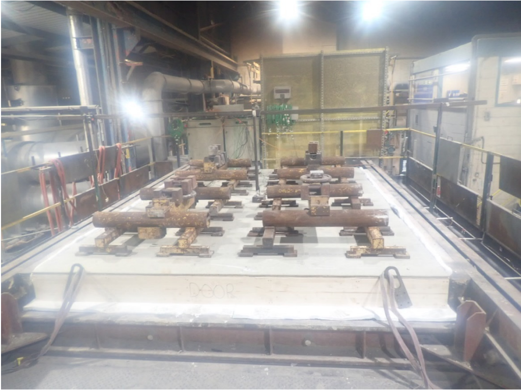
The unexposed face of the floor assembly prior to test
