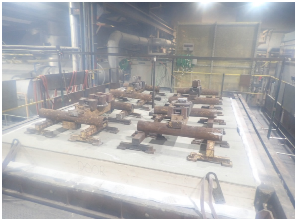
The unexposed face of the floor assembly after 33 minutes of testing
