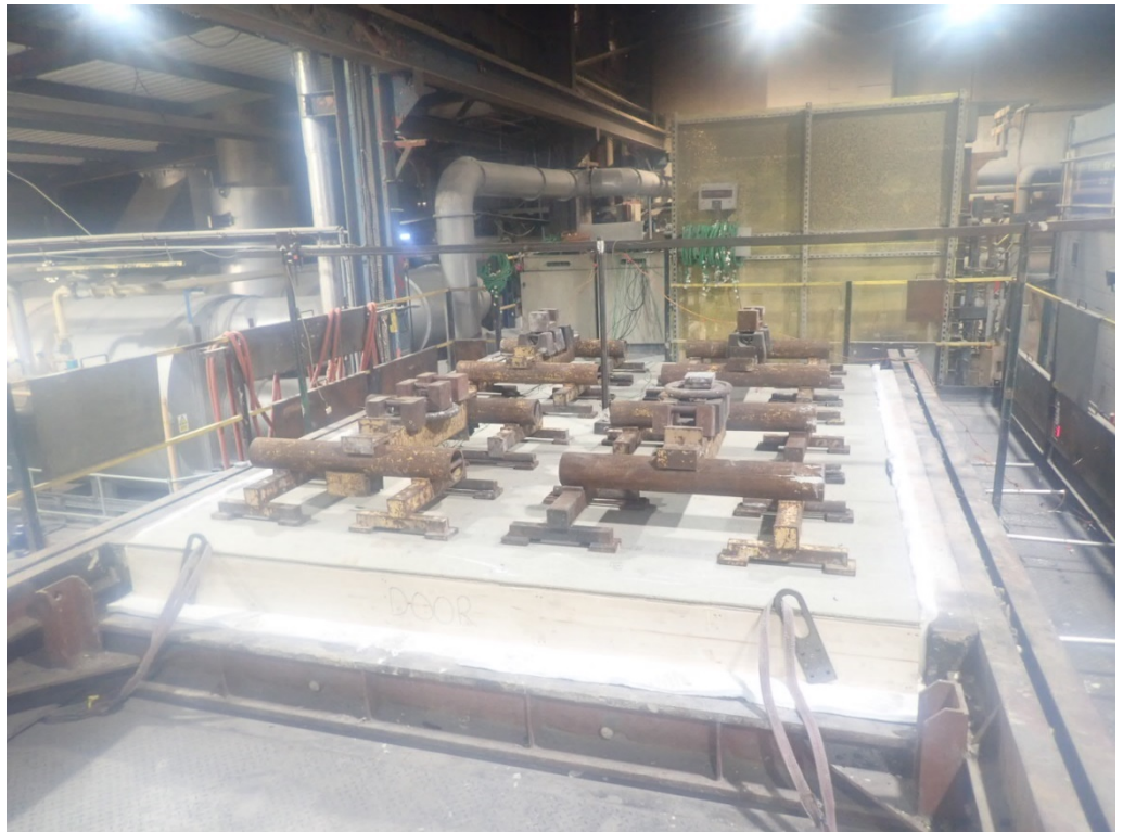
The unexposed face of the floor assembly after 20 minutes of testing
