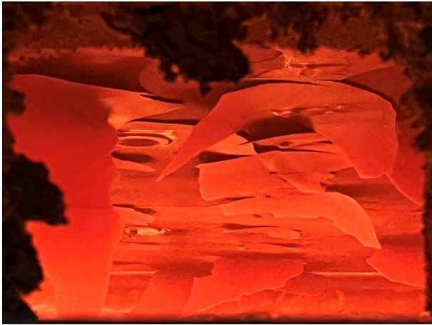
Photo 29: The exposed surface of the specimen after test duration of 25 minutes, large areas of coating of the plasterboard ceiling fell away.
