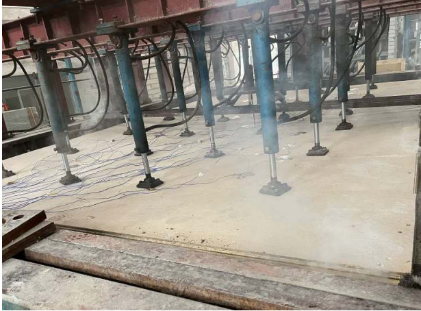
Photo 33: The unexposed surface of the specimen after test duration of 90 minutes.
