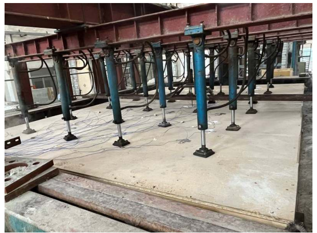
Photo 30: The unexposed surface of the specimen after test duration of 30 minutes.
