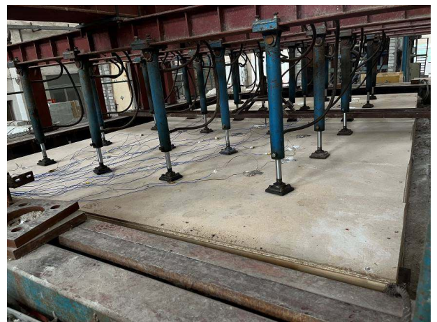
Photo 28: The unexposed surface of the specimen after test duration of 15 minutes.
