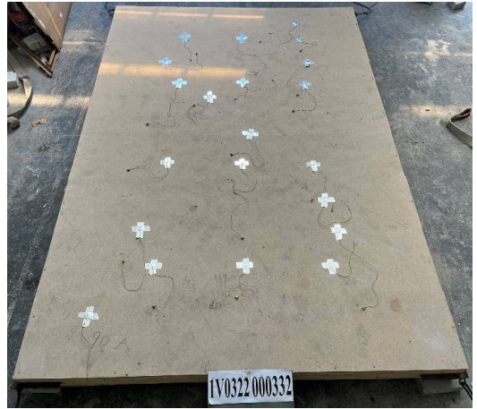
Photo 26: The unexposed surface of the specimen before the test.
