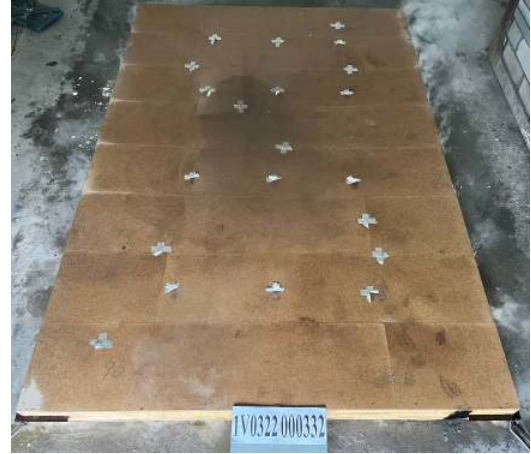
Photo 34: The unexposed surface of the specimen after the test.
