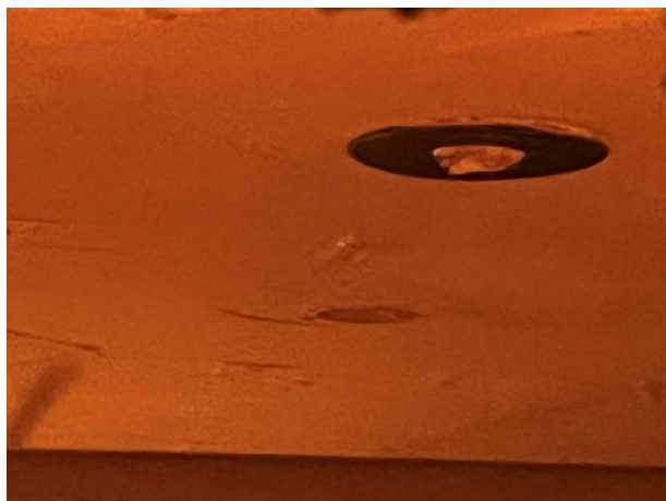
Photo 27: The exposed surface of the specimen after test duration of 3 minutes, showing the lens of specimen was fusing.
