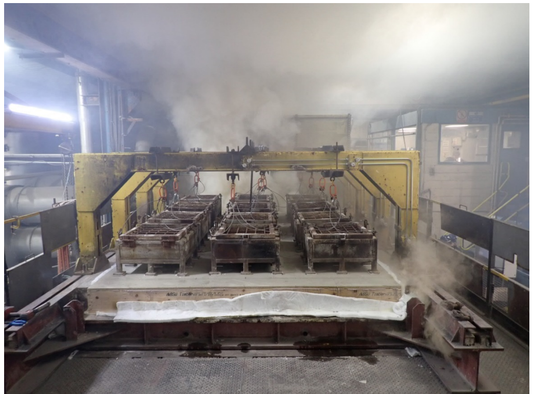
The unexposed face of the floor assembly after 30 minutes of testing
