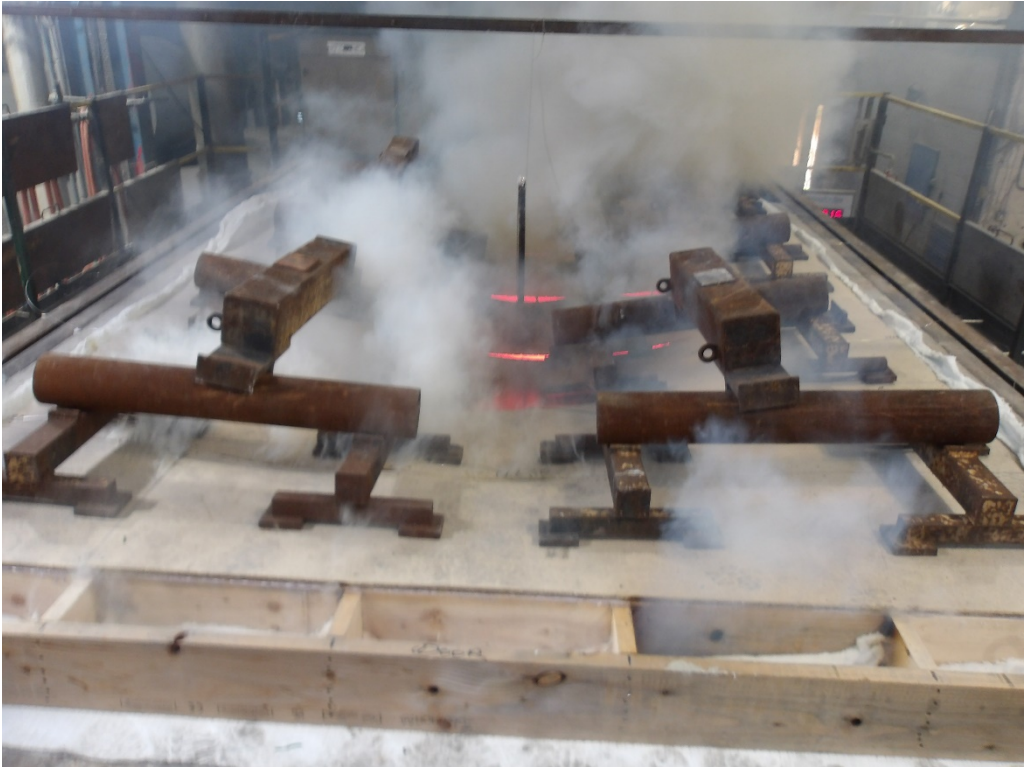
The unexposed face of the floor assembly after 43 minutes of testing
