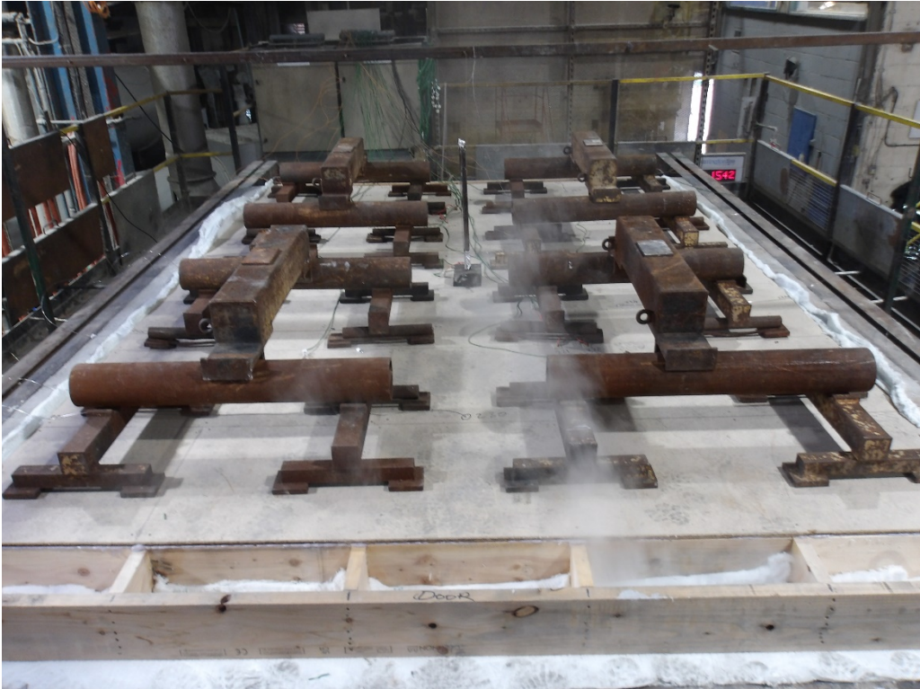
The unexposed face of the floor assembly after 15 minutes of testing
